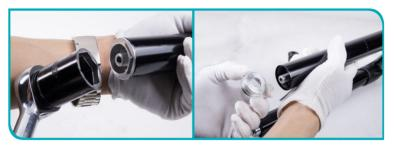
• Use pliers to remove the air spring assembly.
