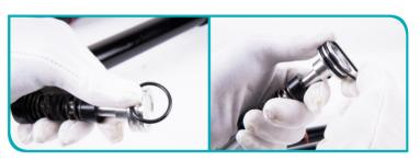
• Apply the grease to the air piston and the spring.
