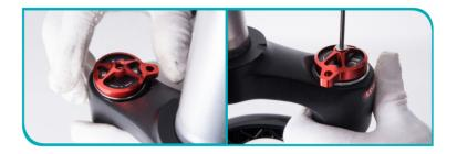
Test the lockout adjuster knob.
