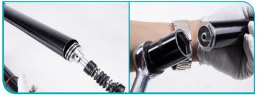
Install and tighten the top cap.
