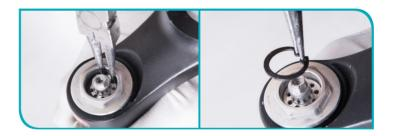
Remove the knob retaining nut, watch out for the tiny balls and the tiny springs.
