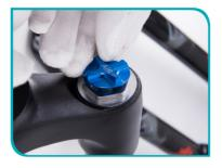
Depress the Schrader valve and release all air pressure.
