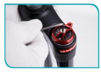
• Remove the retaining ring.
