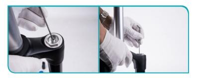
Use the 6mm hex wrench to unscrew the bottom screw.
