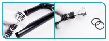
• Apply the grease to the new o-rings and put them back firmly.
