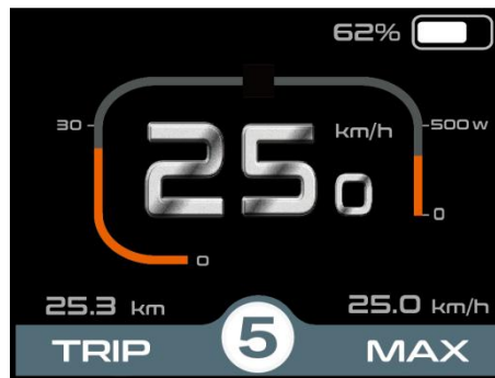
Motor power display interface
