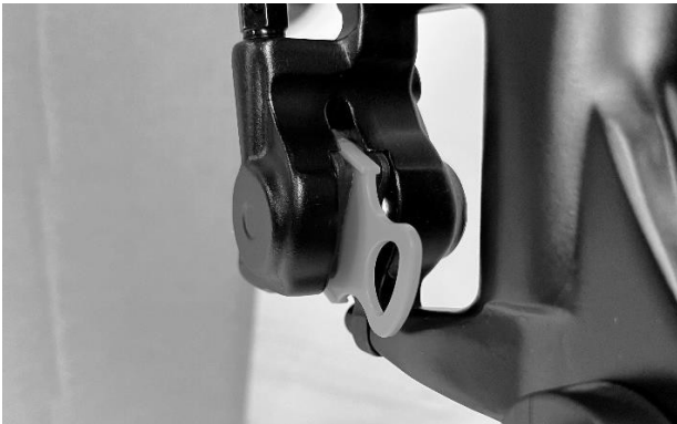
Figure 11 - Transport brake lock
