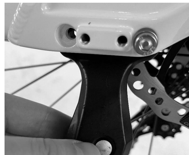
Figure 27 - Bolt holes for the stand mounting
