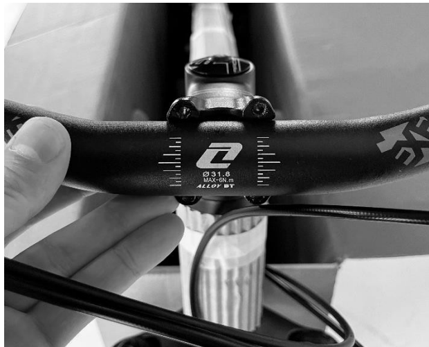
Figure 7 - Centered handlebars in the stem
