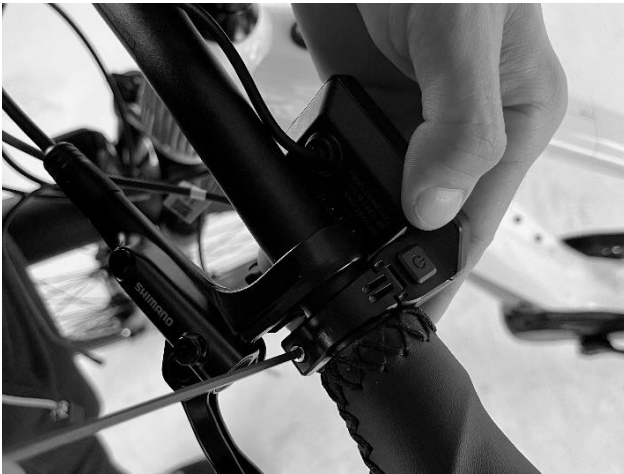
Figure 29 - Correct display position
