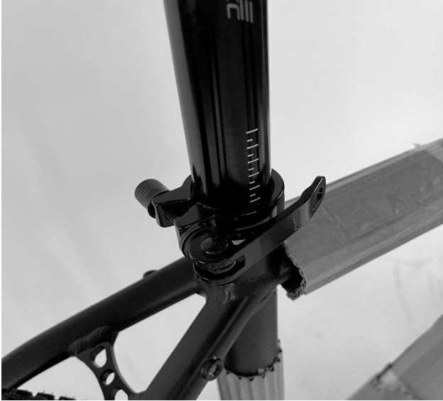
Figure 5 - Setting the desired saddle post height
