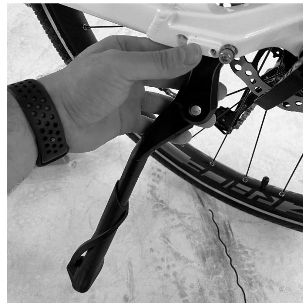
Figure 27 - Bolt holes for the stand mounting
