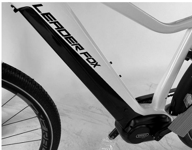
Figure 19 - Electric bike frame with motor and battery installed
