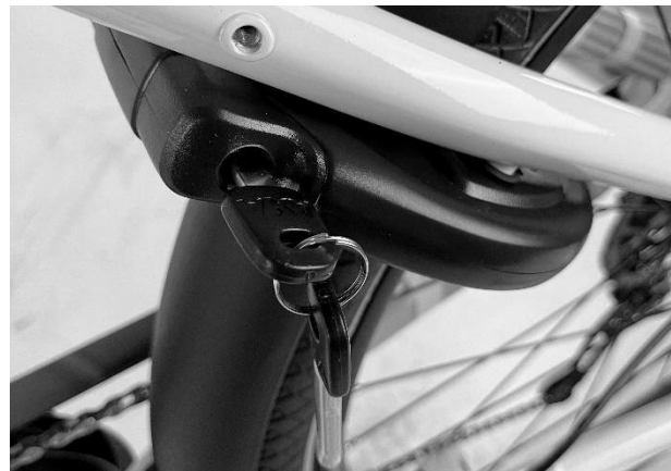
Figure 31 - Integrated wheel lock
