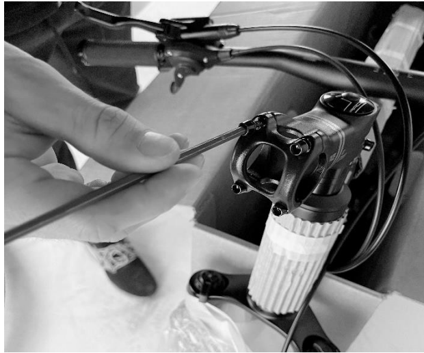
Figure 6 - Loosening the stem bolts
