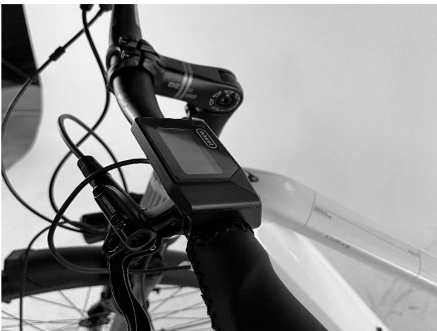
Figure 29 - Correct display position
