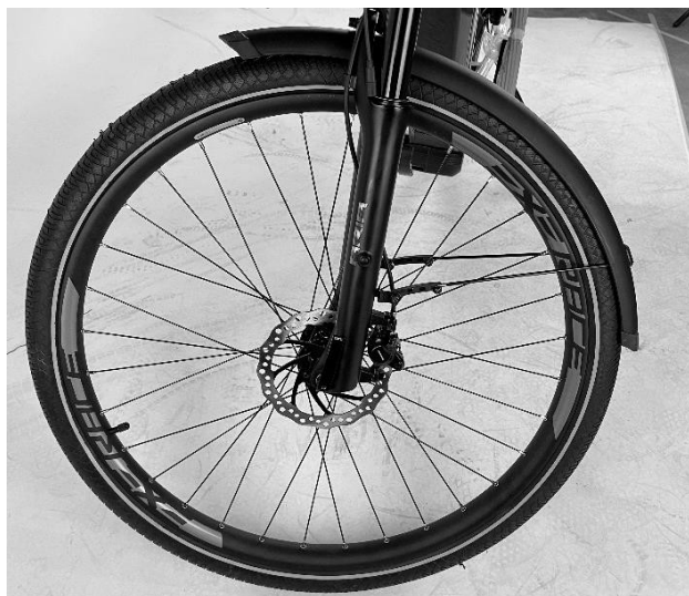
Figure 25 - Correctly installed front mudguard
