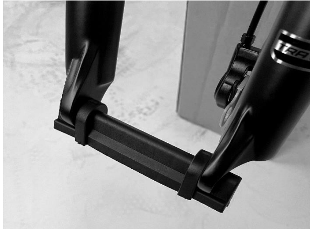
Figure 12 - Wheel axle mounting cap
