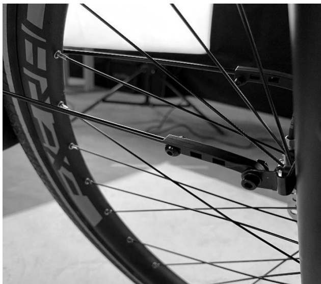
Figure 24 - Attaching the front mudguard to the fork legs
