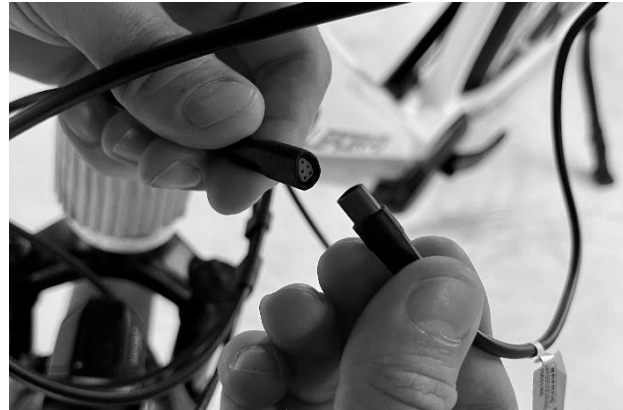
Figure 30 - Connecting the display connector
