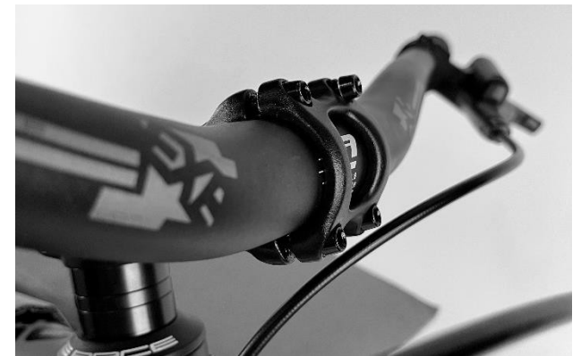
Figure 9 - Correct position of the stem
