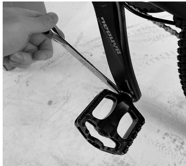
Figure 18 - Tightening the pedal
