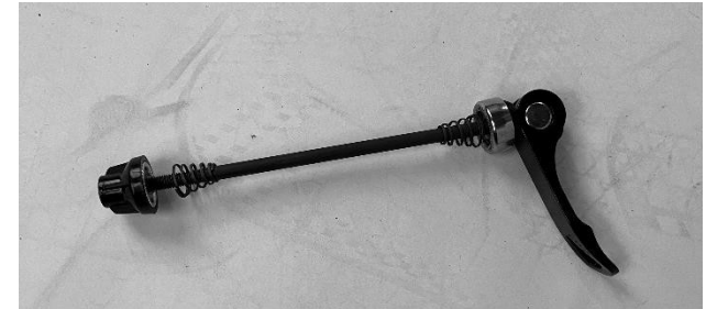
Figure 14 - Quick release pin
