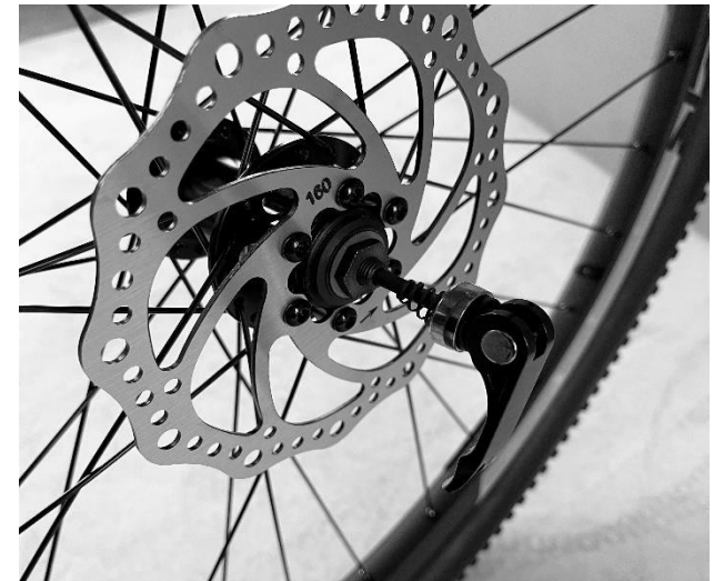
Figure 15 - Inserting the quick release into the wheel axle
