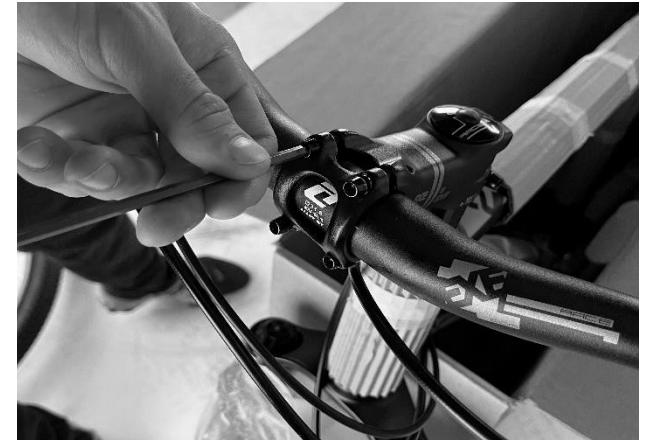
Figure 8 - Tightening the stem bolts
