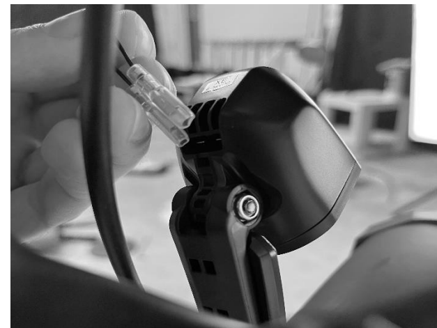
Figure 23 - Front light wiring
