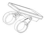
Open the clamps of display and mount on the rubber rings. Place the display on to the handlebar in the correct position.
