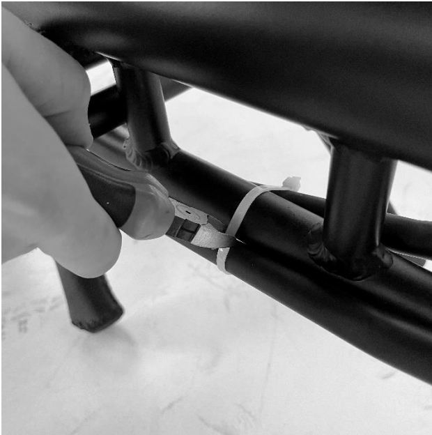
Picture 9 - Tie rod securing tape
