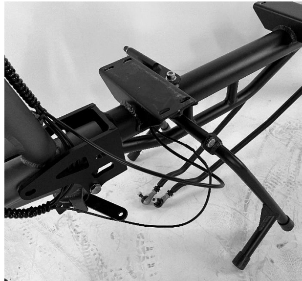
Picture 11 - Bolted joints securing the frame connection
