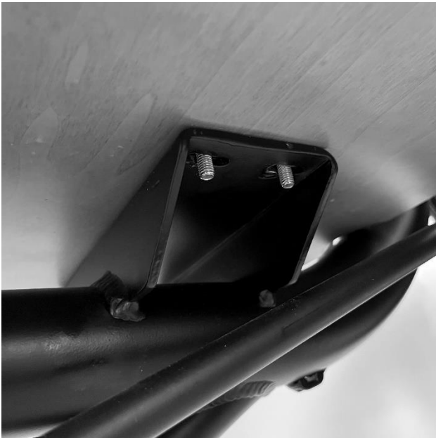
Picture 23 - Cargo box screw connections - bottom side
