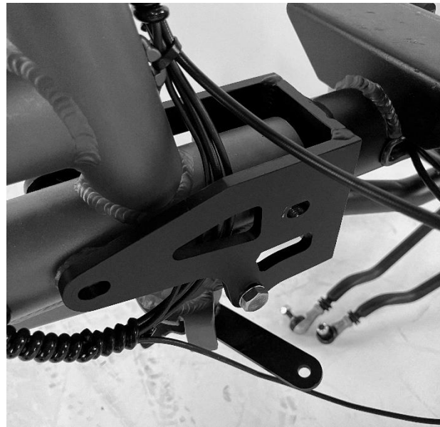
Picture 11 - Bolted joints securing the frame connection
