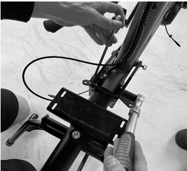
Picture 14 - steering rod bolt connection
