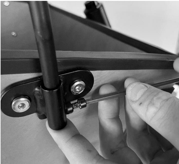
Picture 27 - Securing the sail structure
