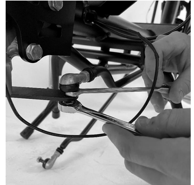
Picture16 - Tightening the screw connection
