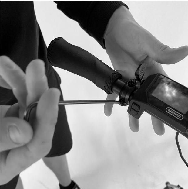
Picture 20 - Mounting the front brake leverbrzdy
