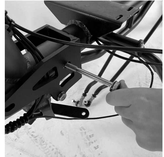
Picture 12 - Screw connections securing the frame connection
