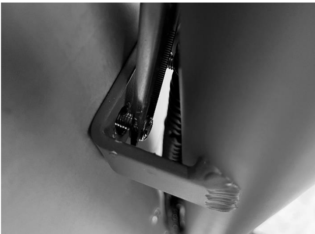
Picture 24 - Cargo box screw connections - attachment to head tube
