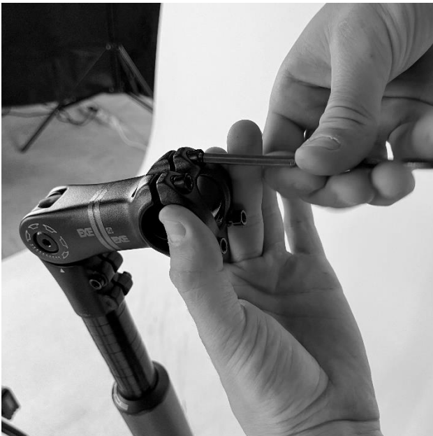
Picture 17 - Loosening the stem bolts
