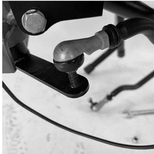
Picture 15 - steering rod bolt connection
