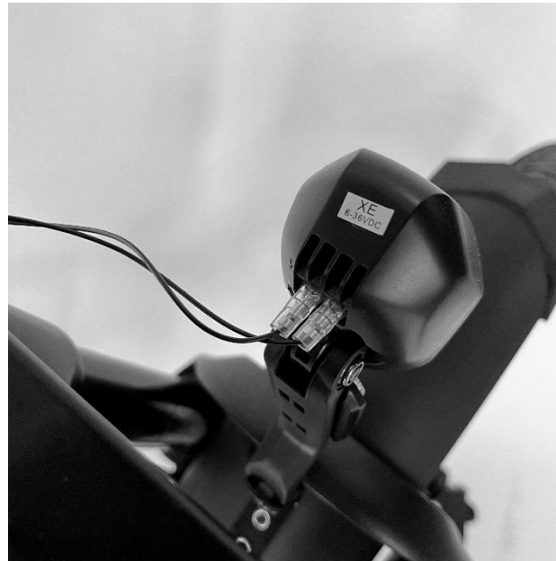
Picture 21 - Front light connected
