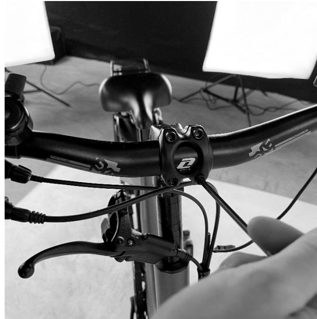
Picture 18 - Tightening the stem bolts
