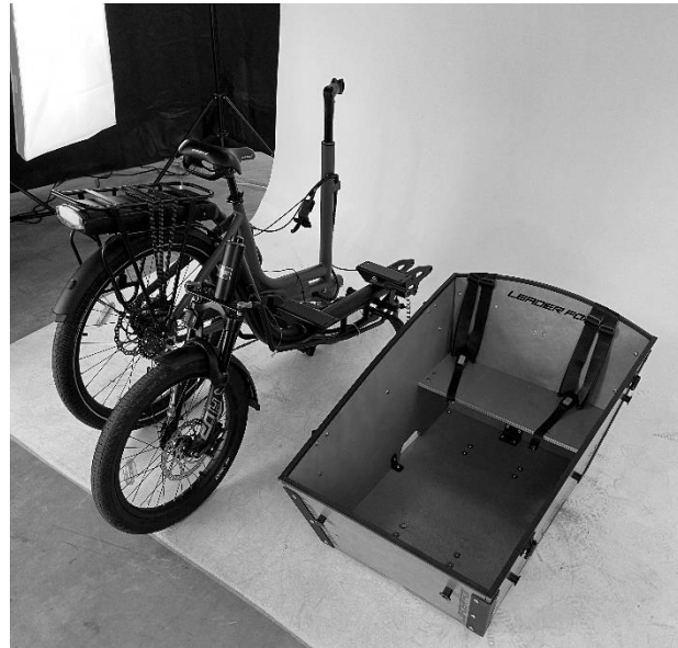
Picture 7 - Removed cargo box
