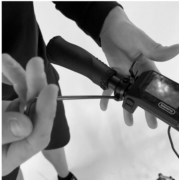
Picture 20 - Mounting the front brake lever
