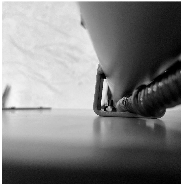
Picture 25 - Cargo box screw connections - attachment to head tube
