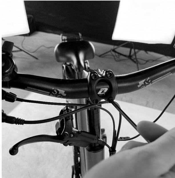
Picture 18 - Tightening the stem bolts
