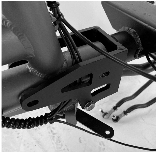
Picture 11 - Bolted joints securing the frame connection
