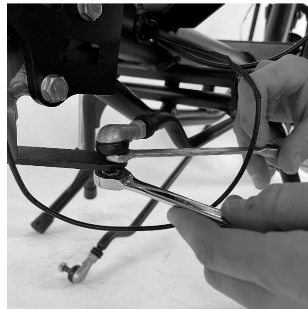
Picture16 - Tightening the screw connection
