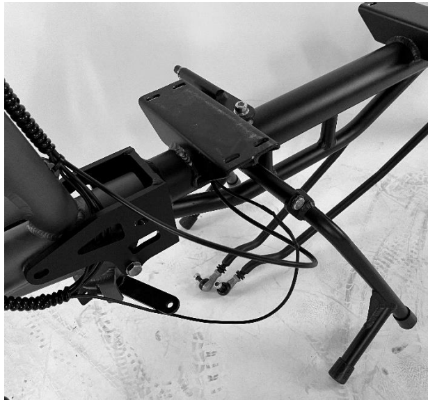
Picture 11 - Bolted joints securing the frame connection
