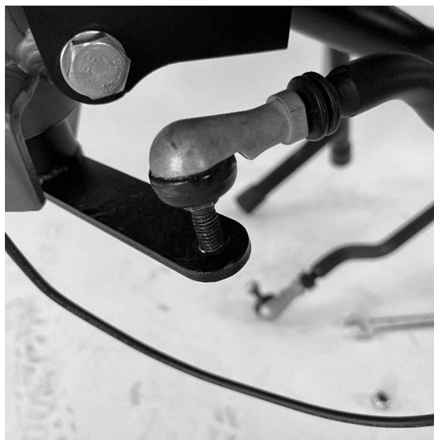
Picture 15 - steering rod bolt connection
