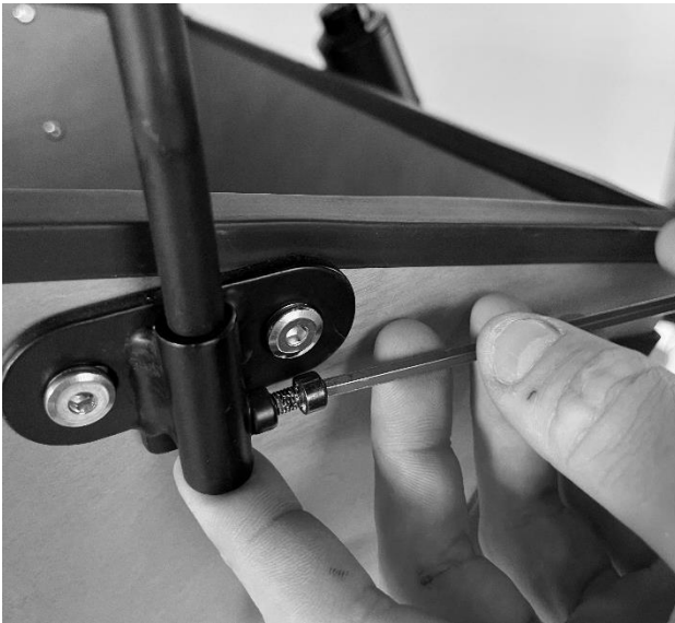
Picture 27 - Securing the sail structure
