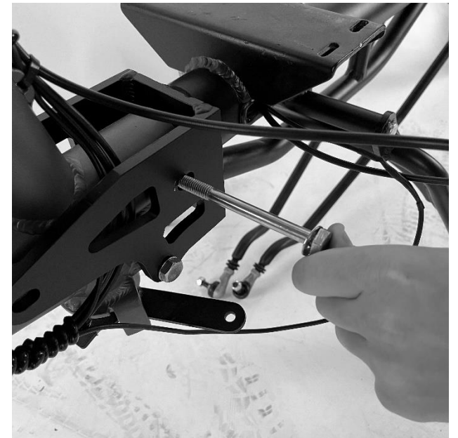
Picture 12 - Screw connections securing the frame connection
