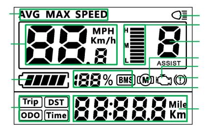
AVG/MAX Speed –indicator of speed mode 00.0 speed Km/h / MPH – indicator of speed unit Battery capacity indicator Trip / DST / ODO / Time – mileage mode Light on indicator 1 assist – level PAS, 0 (off) 5 (max. assist) Error icon Mileage indicator value Trip / DST / ODO / Time
