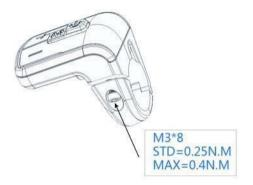
A –controller clamping jaw
