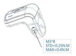
A –controller clamping jaw
