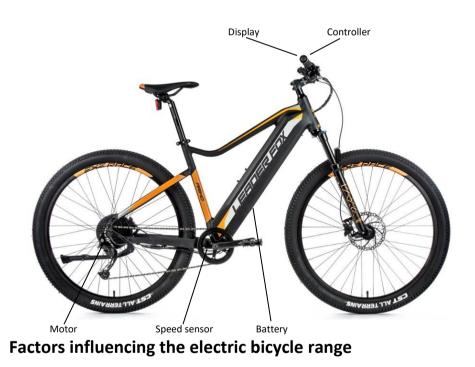
**1. Rolling resistance of the tyres.** Leader Fox e-bikes are fittet with tyres with low rolling resistance and increased resistance to puncture. It is also important that the tyres are inflated properly. Therefor, if the tyres of your electric bicycle are underinflated, the range will decrease.
