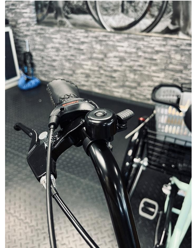
Picture 11 - Correct brake lever position
