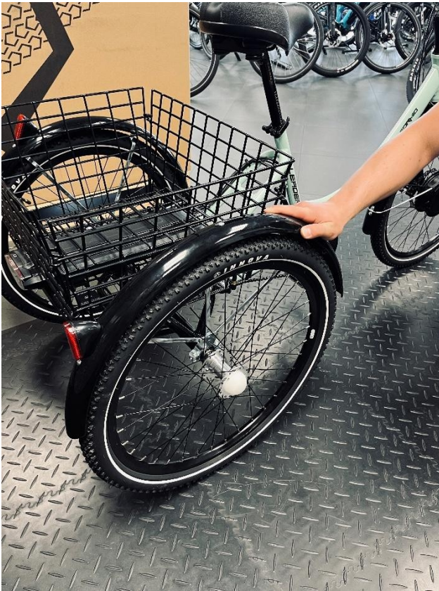
Picture 16 - Aligning the fenders to the correct position
