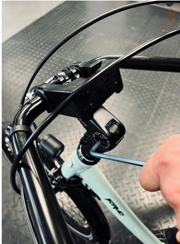
Picture 6 - Loosening the adjustable stem joint
