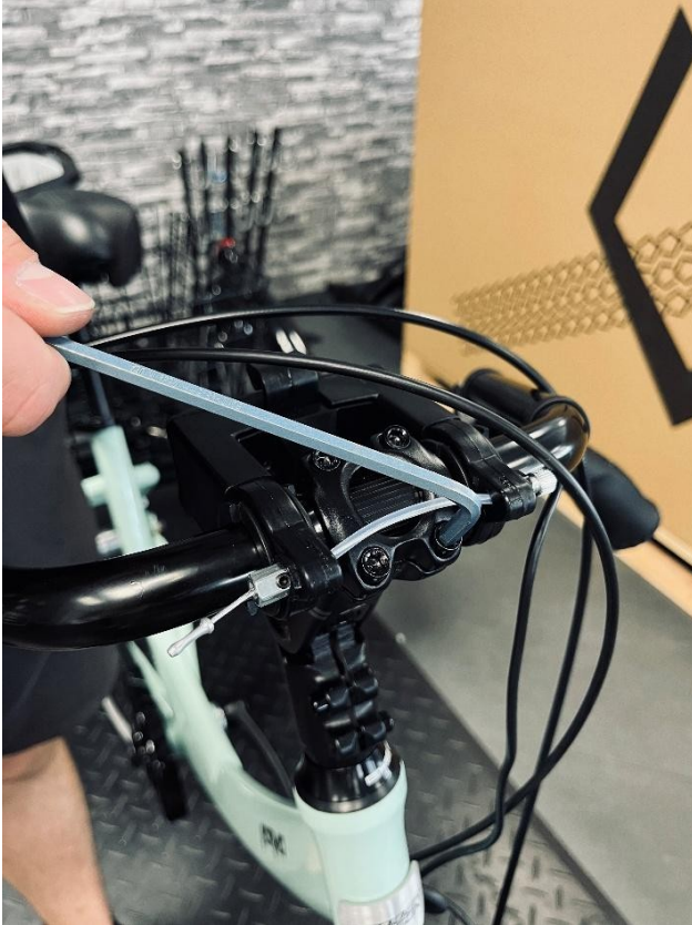
Picture 8 - Loosening the stem socket bolts
