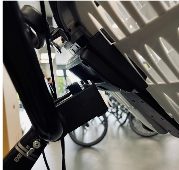
Picture 13 - Fitting the basket to the console
