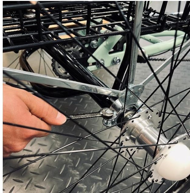
Picture 17 - Tightening the fender bracket bolts
