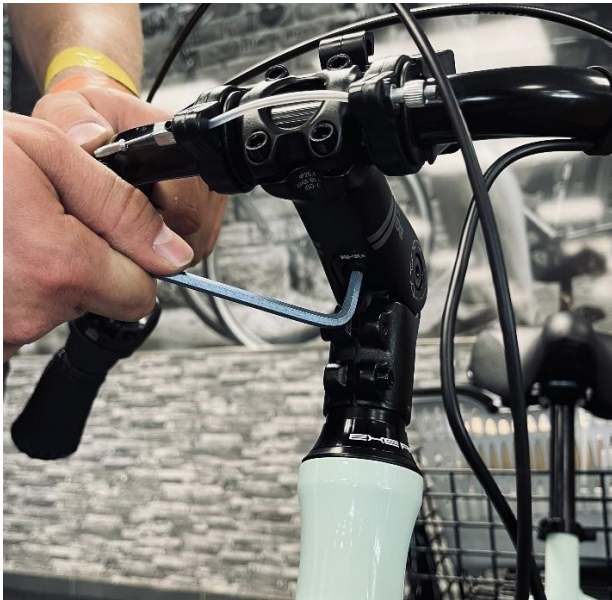
Picture 5 - Loosening the adjustable stem bolt
