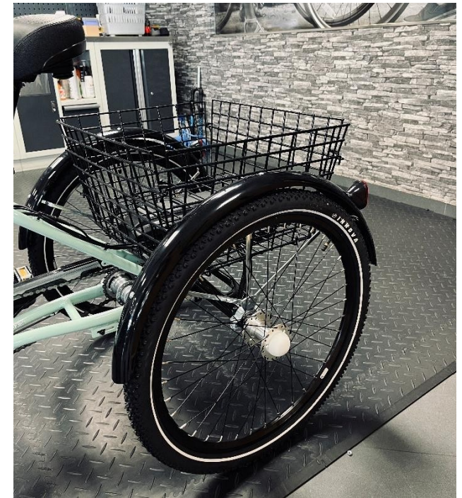
Picture 18 - Correct fender position
