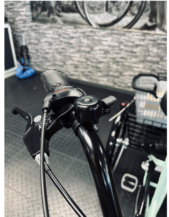
Picture 11 - Correct brake lever position
