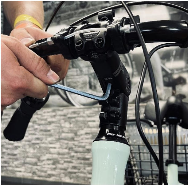
Picture 5 - Loosening the adjustable stem bolt
