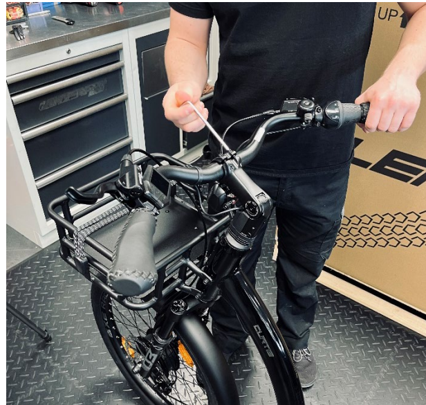
Picture9- Straightening the handlebars
