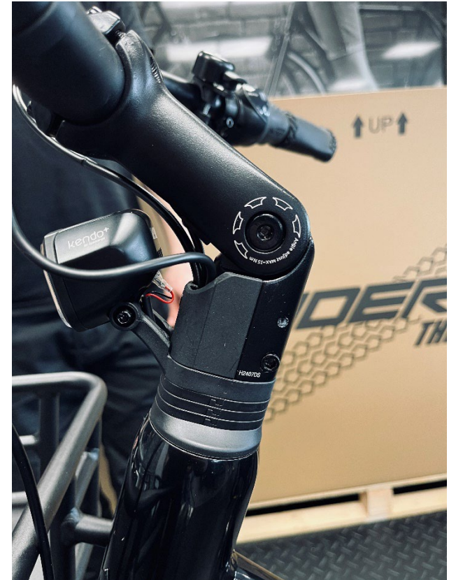
Picture7- Correct stem position
