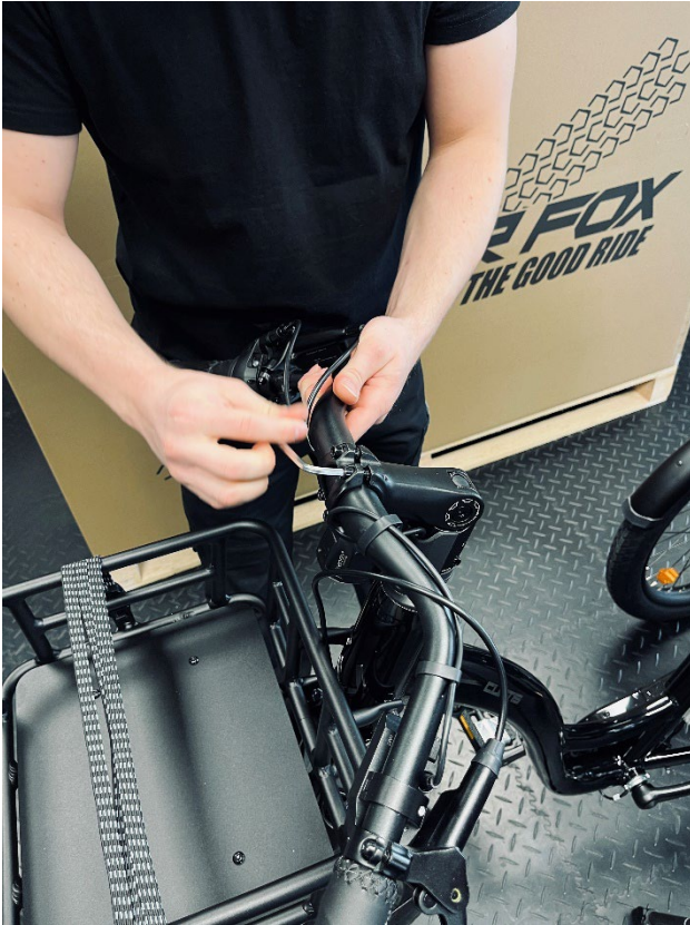
Picture8- Loosening the stem clamp screws
