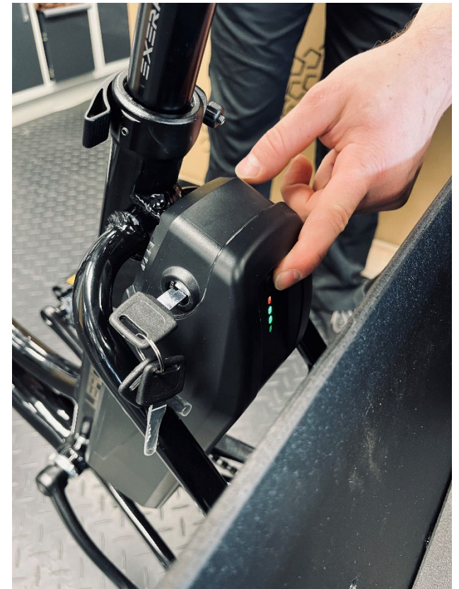
Picture12- Turning on the e-bike battery
