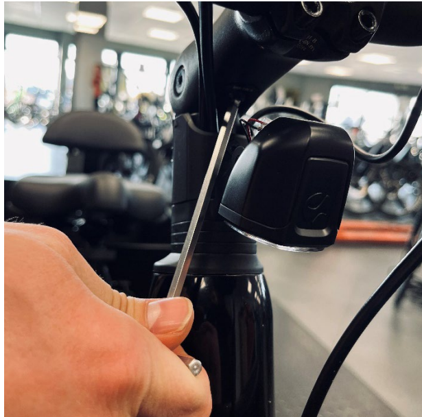
Picture5- Loosening the adjustable stem screw
