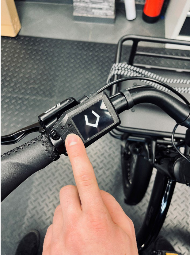
Picture13- Turning on the display
