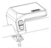
Then place the holding bracket on the underside of the display and tighten it into position with a M3.0\*8 screw. Torque requirement: 1.0 N.m.
