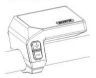
Now connect the Display connector to the EB-Bus connector, ensuring both connectors are kept parallel when pushing firmly together.
