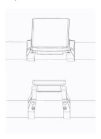
Open the clamp on the control pad and place it in the correct position.
