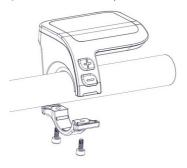
Now connect the Display connector to the EB-Bus connector, ensuring both connectors are kept parallel when pushing firmly together.
