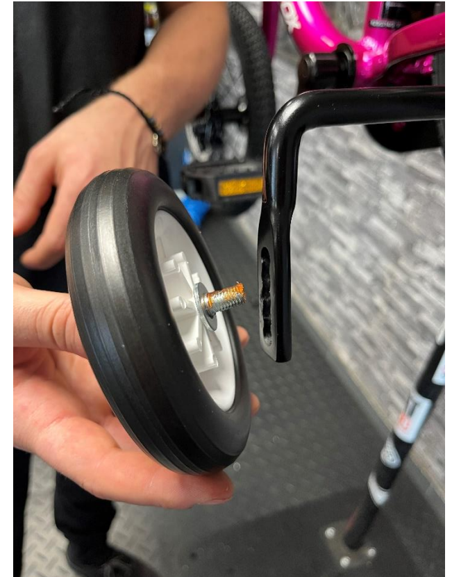
Picture 13 - Screw for fixing the wheel to the structure
