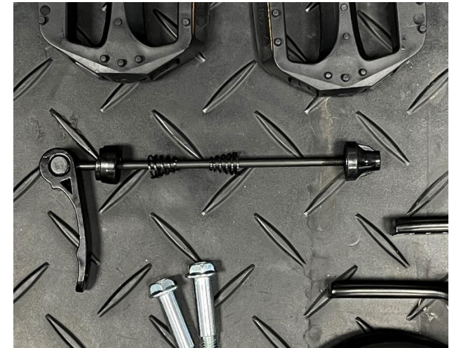
Picture 13 – Front wheel quick-release axle
