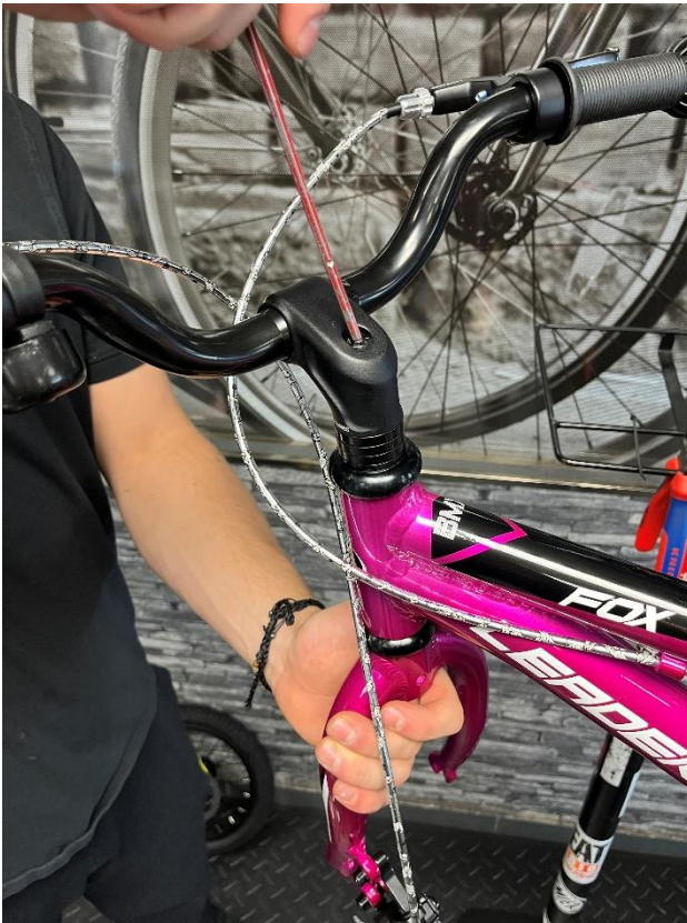
Picture 11 - Assembly of handlebars with stem
