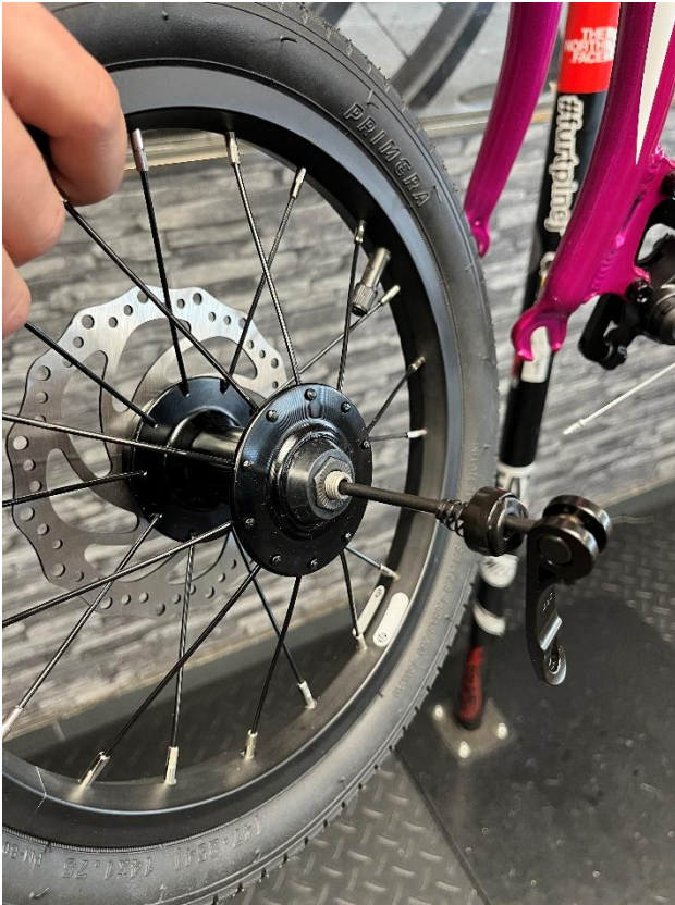
Picture 14 - Quick-release axle inserted in the front wheel hub
