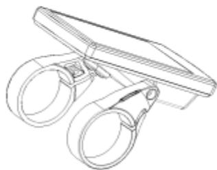
2. Open the clamps of display and mount on the rubber rings. Place the display on to the handlebar in the correct position. Use two M3\*10 screws and M2.5 internal hex wrench to tighten the display. Torque requirement: 1N.m.
