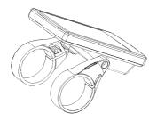
Open the clamps of display and mount on the rubber rings. Place the display on to the handlebar in the correct position. Use two M3\*10 screws and M2.5 internal hex wrench to tighten the display. Torque requirement: 1N.m.
