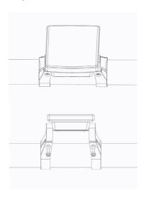
3. Open the clamp on the control pad and place it in the correct position.
