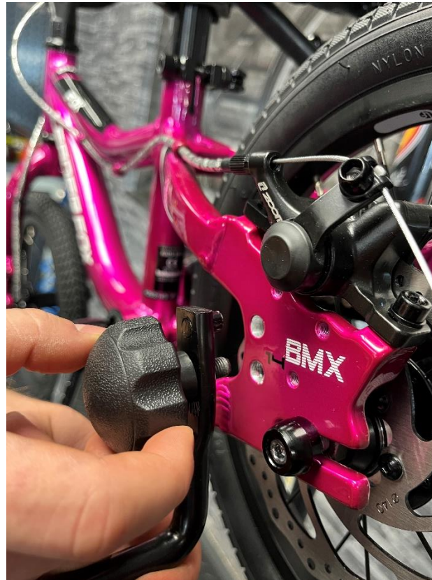
Picture 17 - Assembly of the construction of the additional wheels
