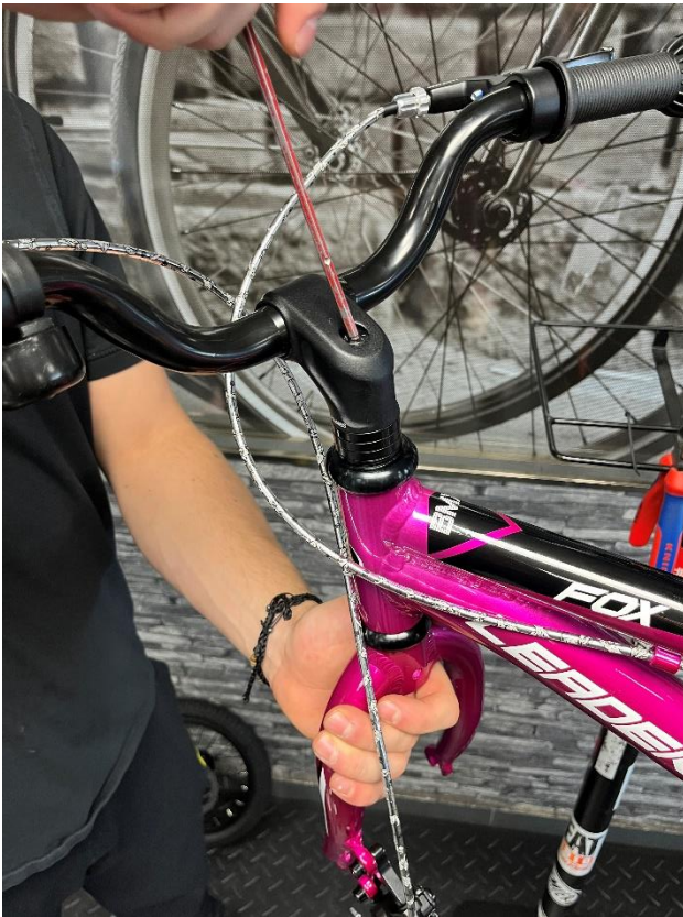
Picture 11 - Assembly of handlebars with stem
