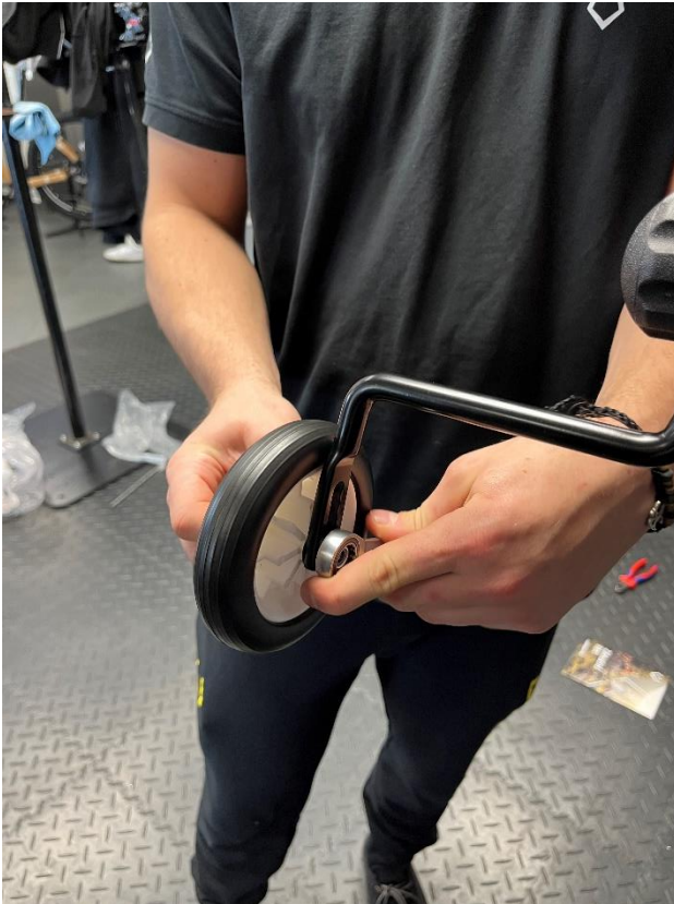
Picture 14 - Securing the nut of the additional wheel
