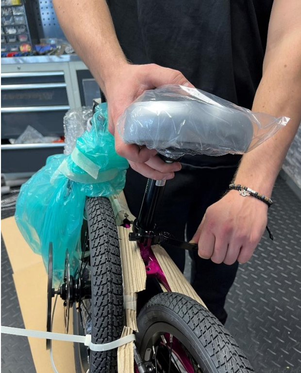
Picture 5 – Inserting the seat post into the seat tube
