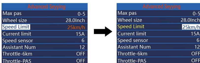
The diagram shows two screenshots of the 'Advanced Setting' menu. In the first screenshot, 'Speed Limit' is set to 25km/h. An arrow points to the second screenshot, where 'Speed Limit' is highlighted in yellow, indicating it is selected. All other settings remain the same.
