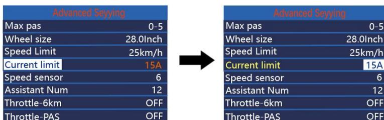
The diagram shows two screenshots of the 'Advanced Setting' menu. In the first screenshot, 'Current limit' is set to 15A. An arrow points to the second screenshot, where 'Current limit' is highlighted in yellow, indicating it is selected. All other settings remain the same.
