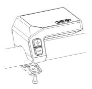
Now connect the Display connector to the EB-Bus connector, ensuring both connectors are kept parallel when pushing firmly together.
